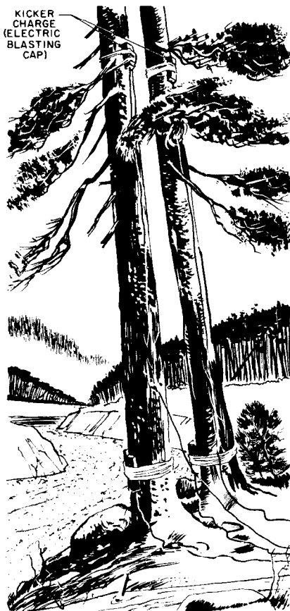
Figure 94. External timber-cutting charge.
